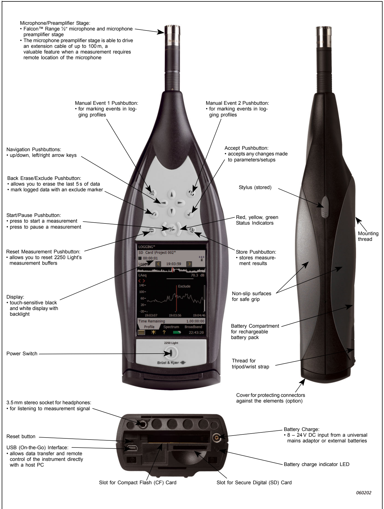
Fig. 1 Key features of 2250 Light
